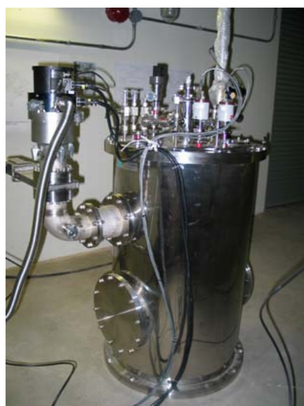
LH2 Absorber Cryostat – KEK
