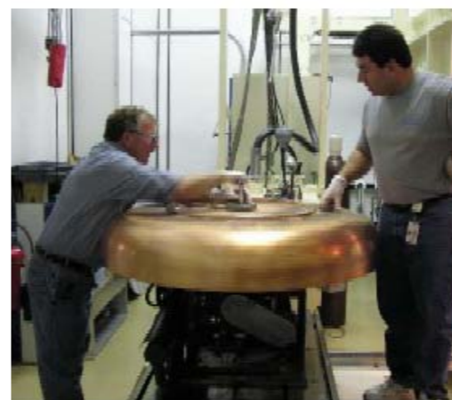
201 MHz half-shell ebeam welding of Stiffening – JLab
