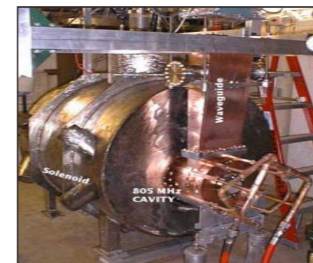
5T Cooling Channel Solenoid – LBNL & Open Cell NCRF Cavity operated at Lab G – FNAL
